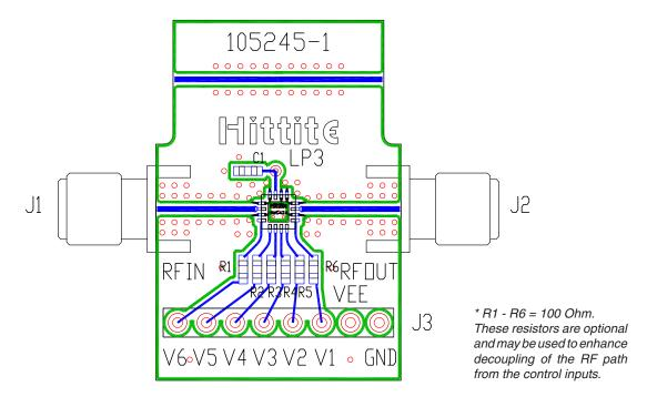
The circuit board used in the final application should use RF circuit design techniques. Signal lines should have 50 ohm impedance while the package ground leads and exposed paddle should be connected directly to the ground plane similar to that shown. A sufficient number of via holes should be used to connect the top and bottom ground planes. The evaluation circuit board shown is available from Hittite upon request.
